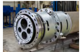
revamped M.A.S. burner
