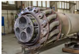
existing M.A.S. kiln burner
