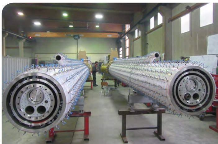
Figure 1. M.A.S./6/KO.SO.X in the Unitherm workshop before refractory installation.
