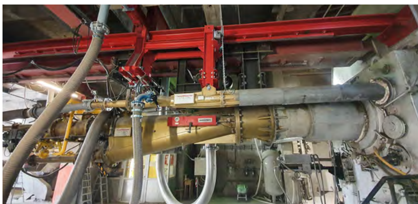
Figure 4. The satellite burner was installed on a monorail beside the main burner.
